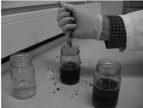
Picture 4.1 Preparation of the specific 1:2 volume extract. Sufficient field-moist soil is added to two parts of water so that the volume is increased with one part
