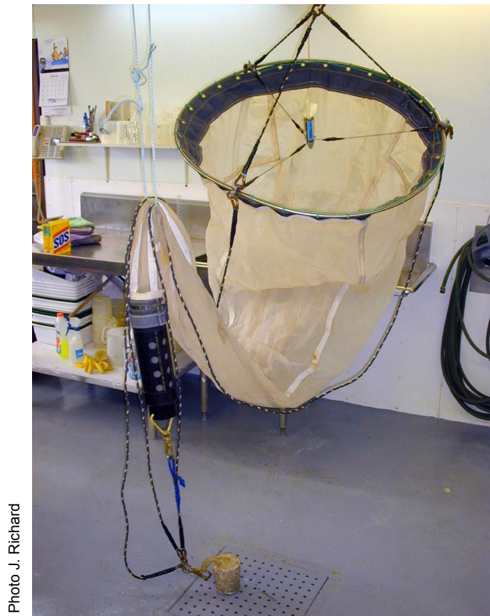
Figure 6. Plankton net for vertical tows.
