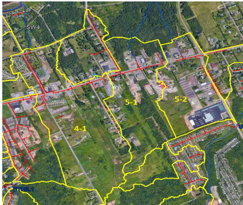
Figure 25. Example watersheds showing relative extent of development and impervious cover. Watershed boundaries in yellow, stormwater pipes in red.
