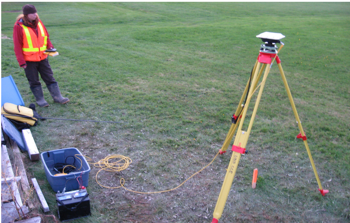
Figure 3. GPS base station #1. Note wooden stake beneath the antenna. The blue bin contains the yellow GPS receiver and a DC-AC inverter eventually replaced by a direct DC connection.
