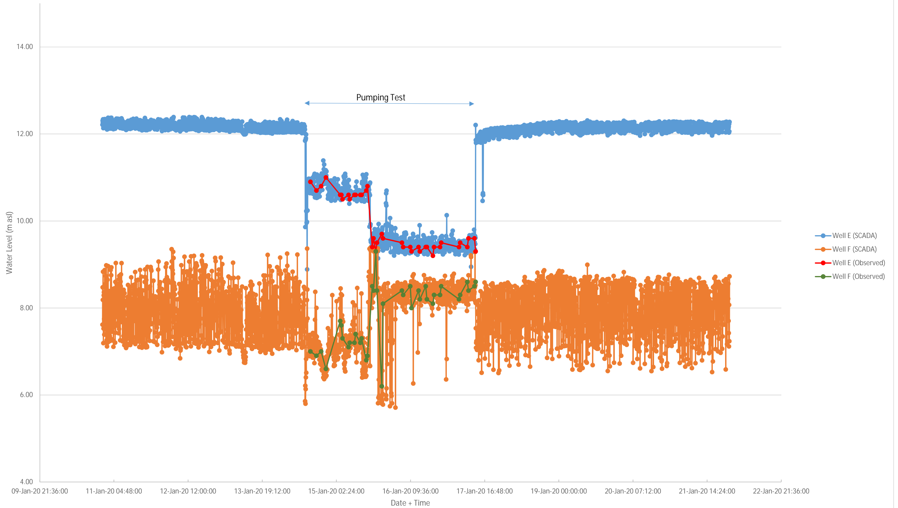
Figure 2: Water Levels in Wells E & F
